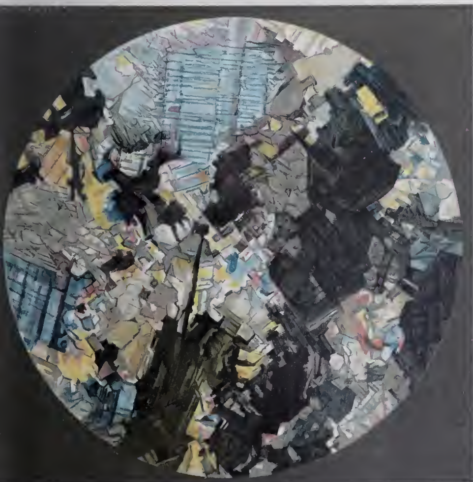
Thin section, in polarized light, of a Rock near Germantown, Philadelphia, magnified 35 diameters.
